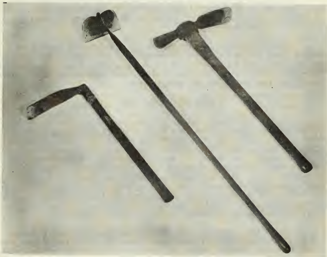
Figure 3.--Typical tools used in grass release of coniferous plantations. Light grub hoe (on left), hoe, and mattock (right).
